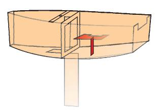
9. Insert mast and rudder tube.
