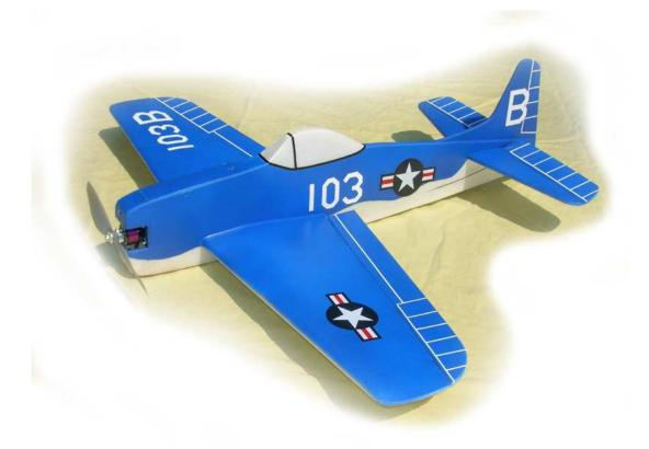
Specifications Wing Span: 32 inches Wing Area: 210 in<sup>2</sup> Fuselage Length: 26 inches Weight (ready to fly): 11 to 13 oz. Wing Loading: 7.5 to 8.9 oz/ft<sup>2</sup>
