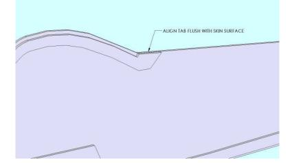
NOTE: The top front doubler needs to be positioned 3 mm from the edge of the skin. An alignment tab is provided at the rear of the part to ensure proper alignment.
